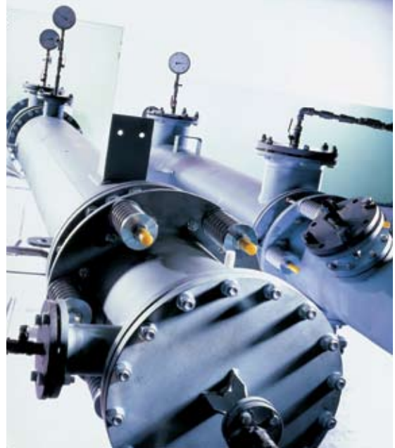
Heat exchanger during pressure testing
