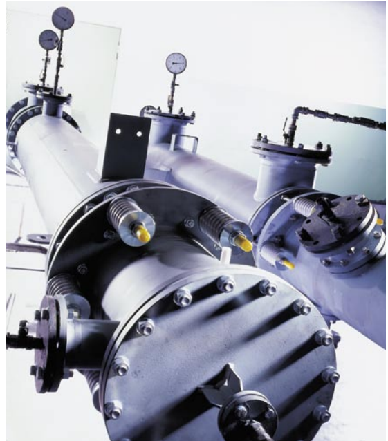
Heat exchanger during pressure testing
